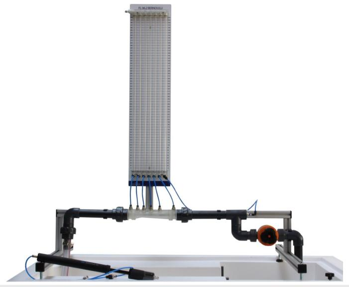
The FL 06.2 equipment is a simple equipment in which to study in depth the Bernoulli equation and its proof.
