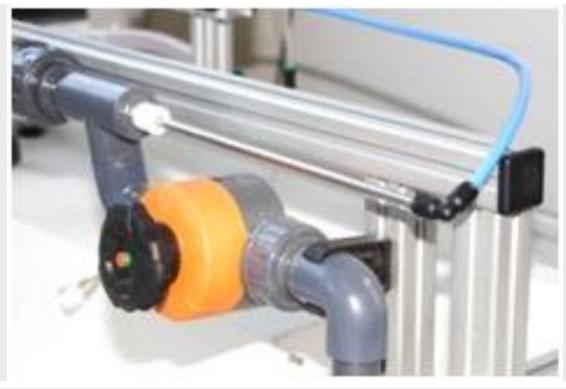
For the study of the static, dynamic and total pressures, the equipment has a pitot tube, whose position within the venturi can be varied.
